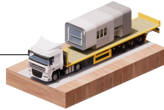
2. Transporting them on a trailer
